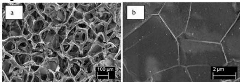
Fig 1: SEM image of a) interconnected 3D graphene, b) wrinkles and ripples on the surface.
