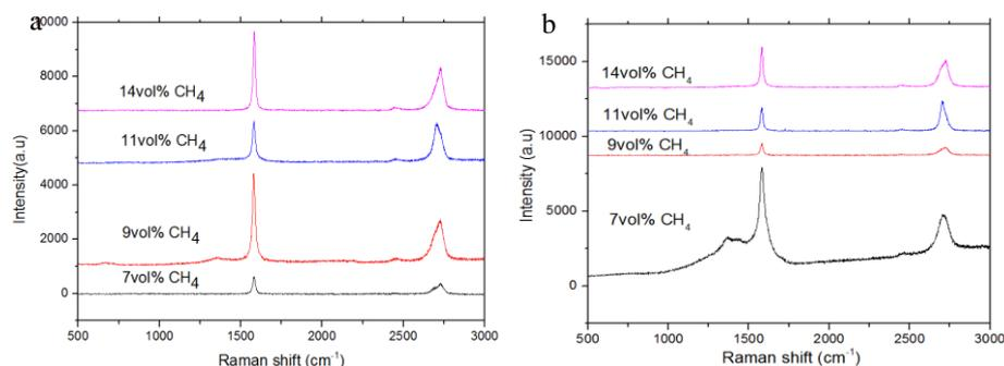
Fig 2: Raman spectrum for varying concentration of  $\text{CH}_4$  at a) atmospheric pressure b) low pressure.
